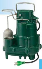
This model is constructed of the same heat-dissipating cast iron with powder coated epoxy finish, providing maximum pumping performance under the most extreme conditions. With Zoeller's cool run design, the hermetically-sealed, oil-filled motor and non-clogging vortex impeller add up to a
